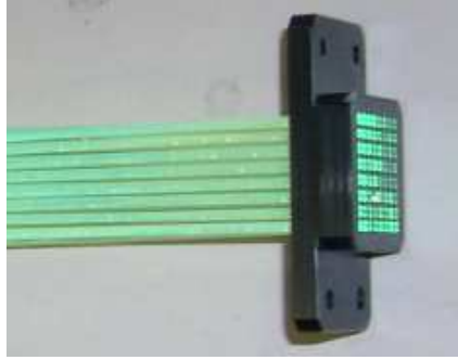
Figure 3.5: Fibers in 8 \times 8 configuration, ready to be aligned with face of MAPMT.
