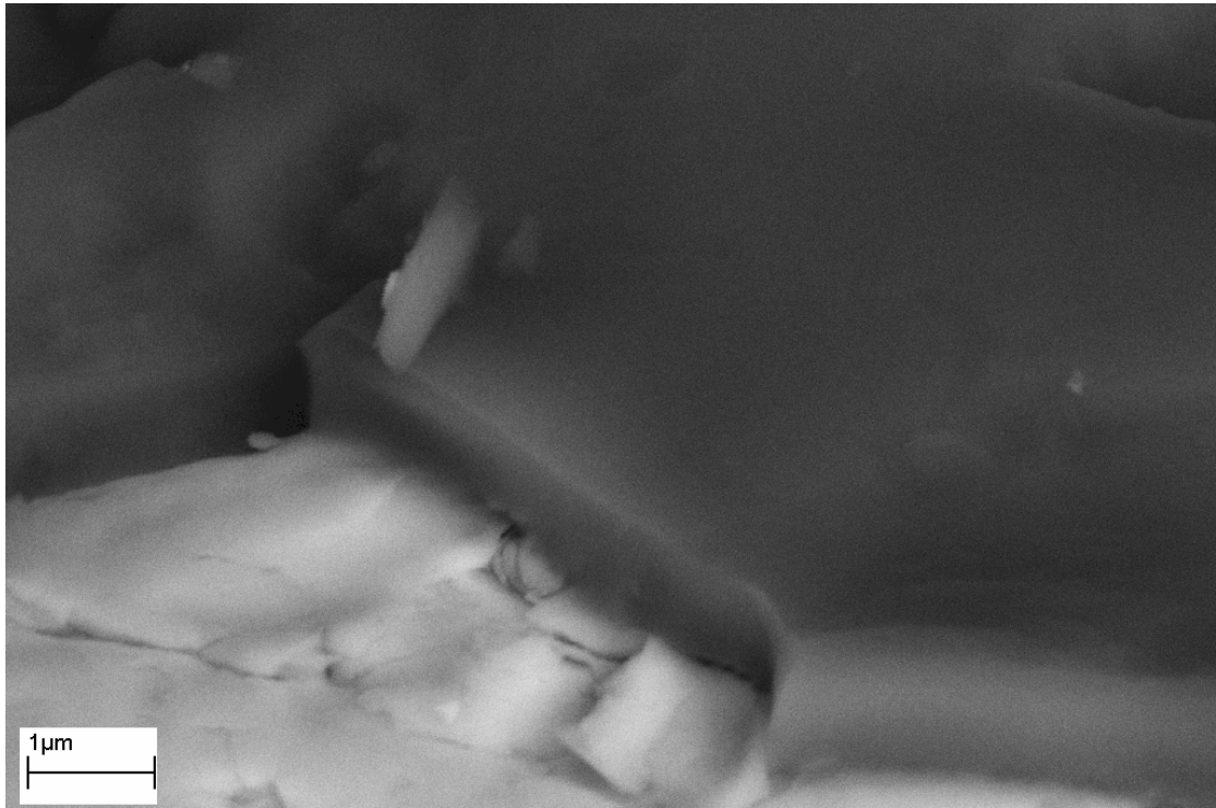
Figure 4.6. BSE of scratch tested specimen. The specimen was tilted 45 degrees. The dark region (low z-contrast) is the SiC film, the bright region (high z-contrast) is the HK40 substrate [9].
