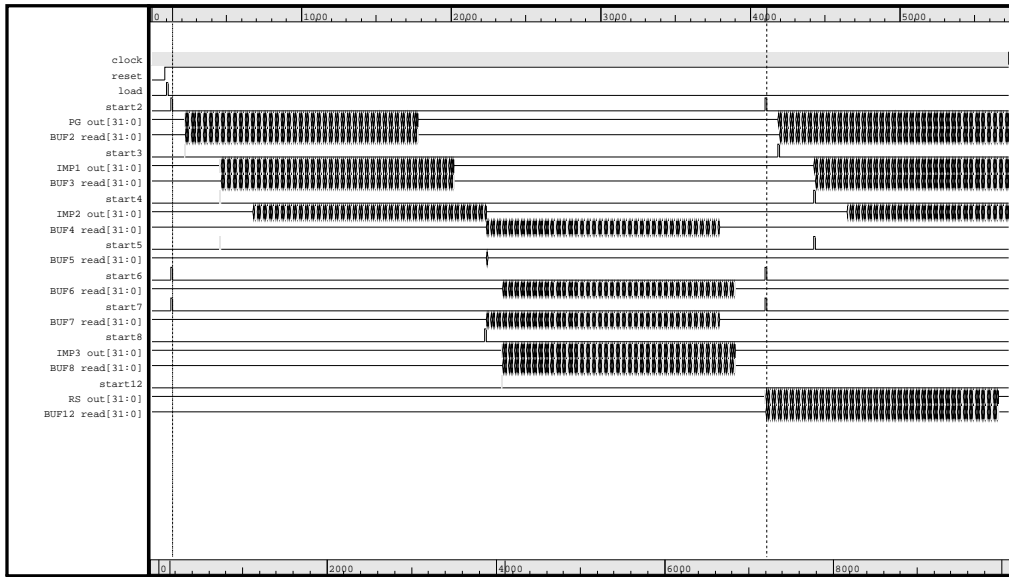
Figure 5.10: Timing diagram of SIRF. The vertical lines indicate the start of the iterations. The diagram illustrates buffer activity.
