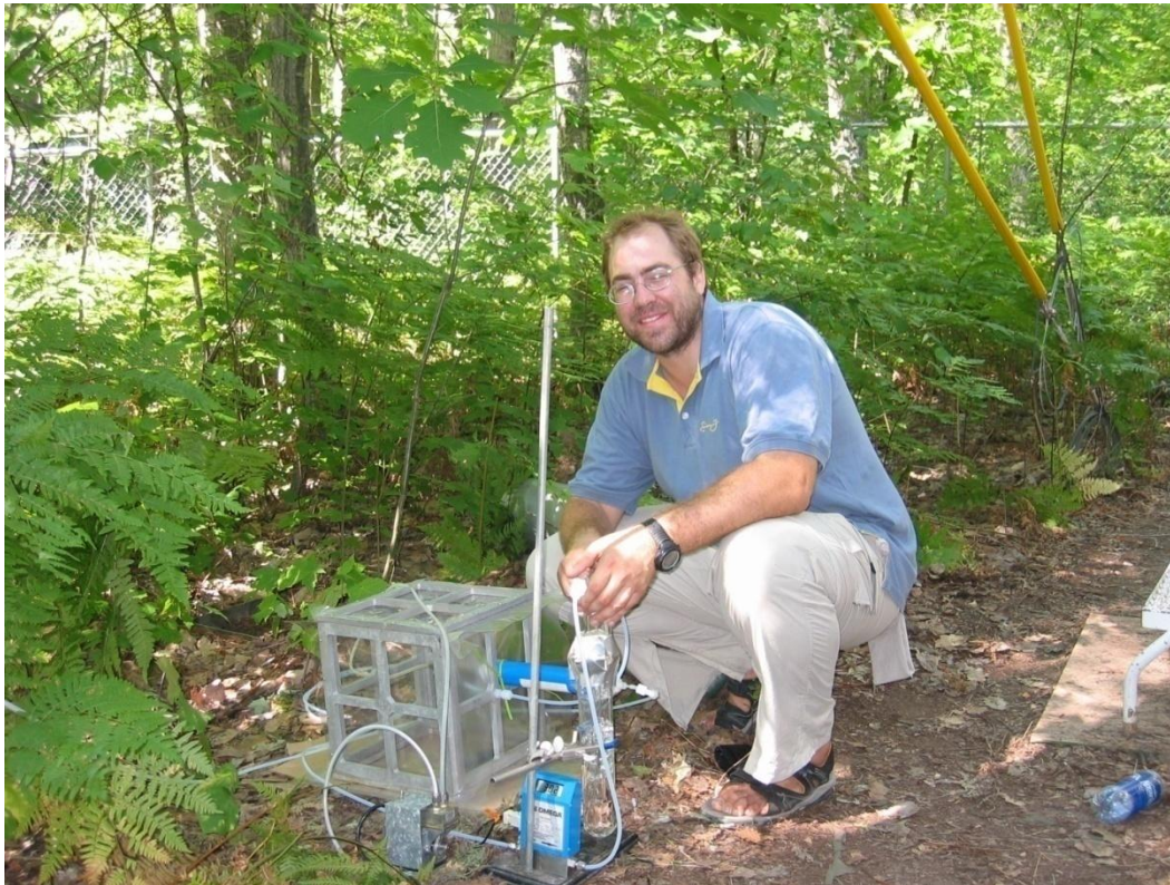
Figure 52: Making soil flux measurements of volatile organic compounds near the PROPHET tower in Northern Michigan, summer 2005.
