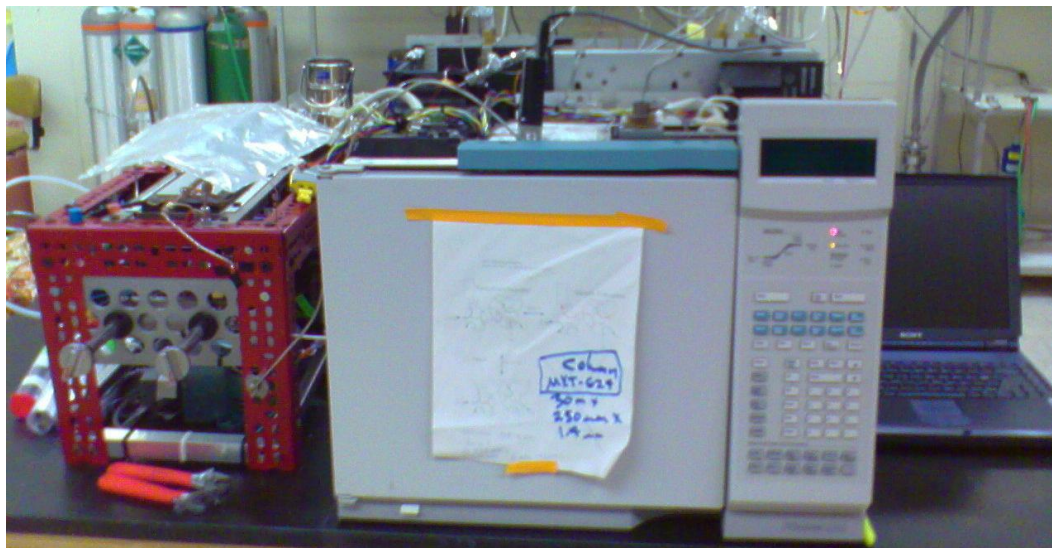
Figure 10: Picture of the GC-FID with custom built VOC preconcentration system.
