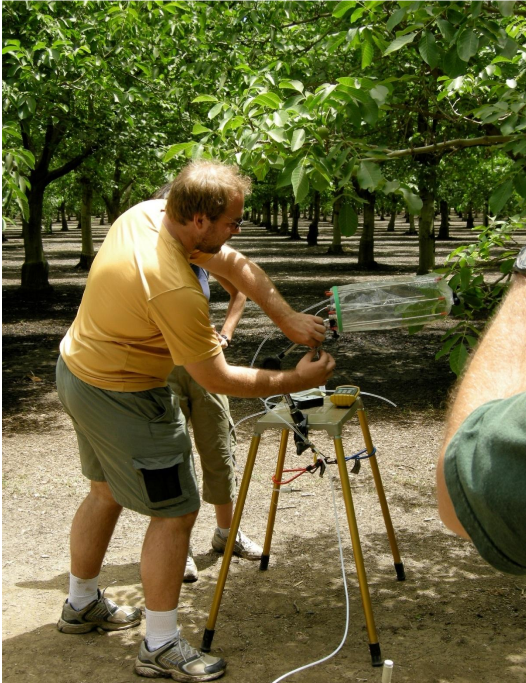
Figure 56: Measuring the emissions of VOCs from a walnut branch during CHATS.
