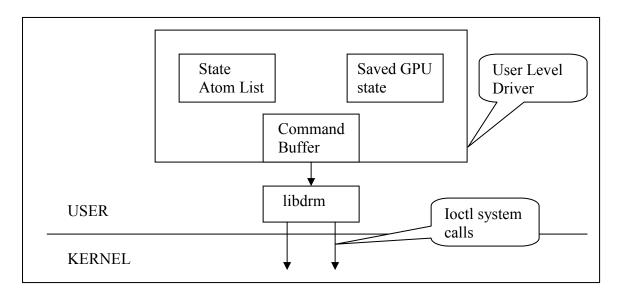
Figure 2 : User Level GPU Driver
