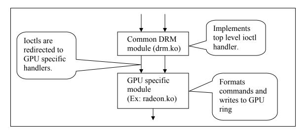
Figure 3: Kernel level GPU Driver
