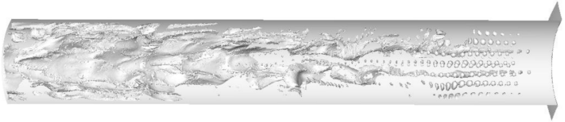
Figure 3.7: The surface of cavitation zone inside the nozzle at steady state. The nozzle inlet is on the right side.
