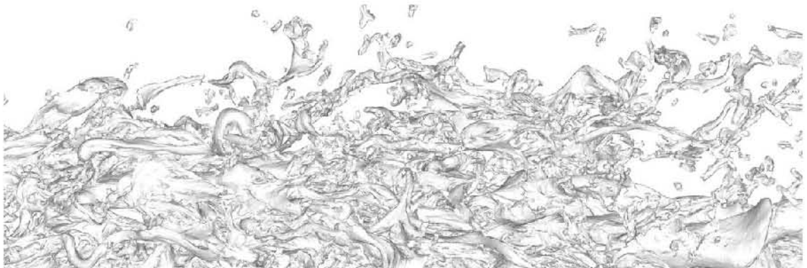
Figure 3.11: The jet interface at the tip of the jet at We = 5 \times 10^4 .
