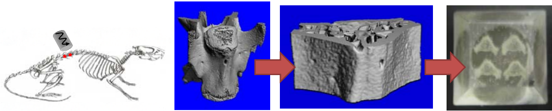
Figure 4.1: An approximately 2mm transverse slice(center) was removed from the center of the L5 vertebra (left) using a water irrigated wafer saw. The samples were dehydrated for 24 hrs in 100% ethanol and embedded in a weakly exothermic epoxy resin (Epothin™, Buhler Inc.). Each sample was then polished to a final surface roughness of 0.05 \mu m (right).
