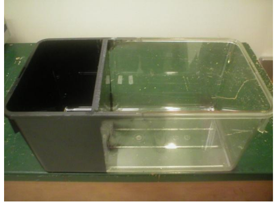
Picture 2 shows the light/dark box. During testing, the dark side of the box is covered by a lid.
