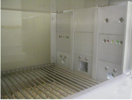
Picture 1 shows the front panel of the operant chamber. To the right and left are the 2 nose-poke ports, and in the center is the reward well.
