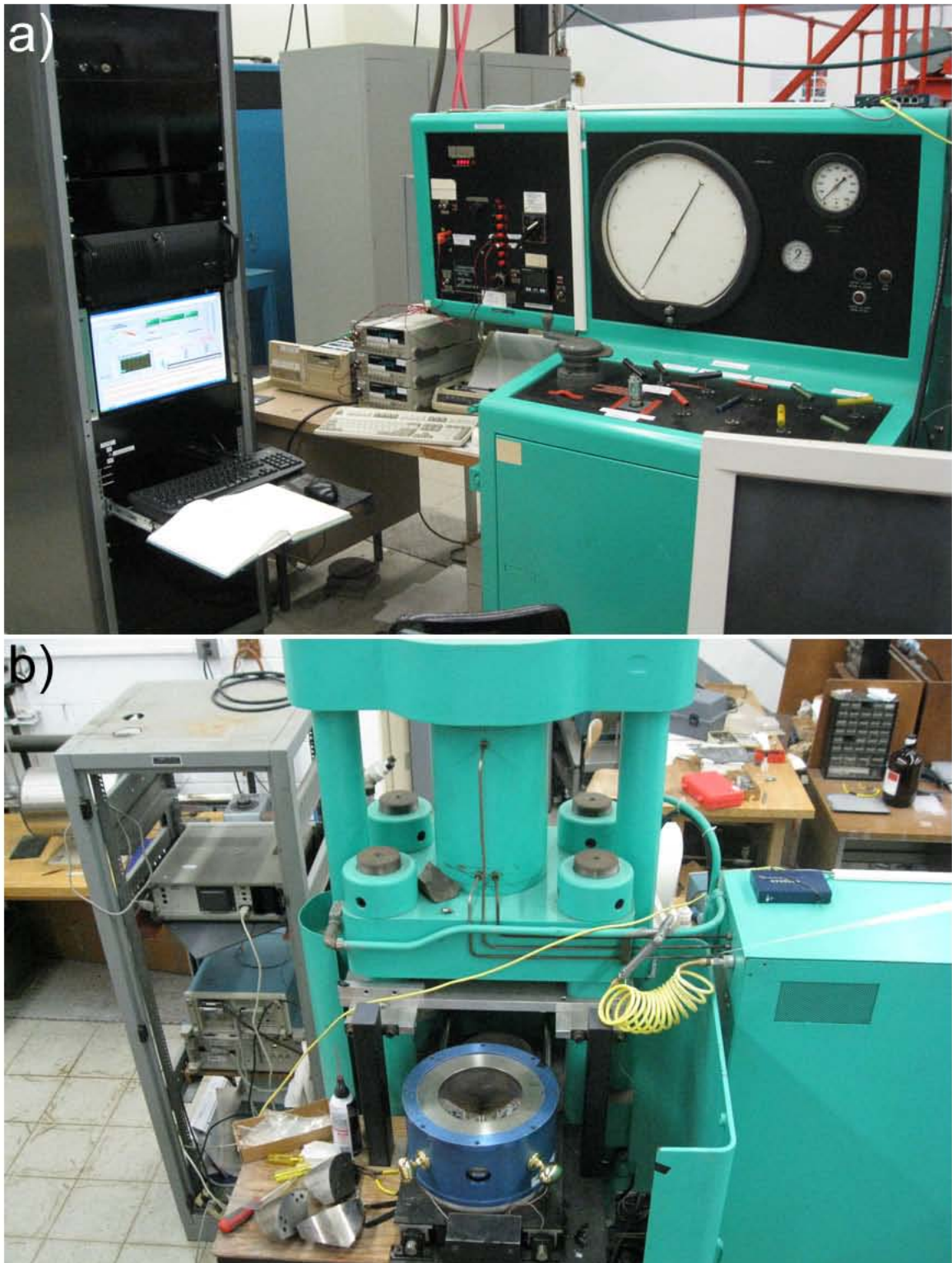
Figure 2.1.1. The Kennedy Press (USCA-1000): 1000-ton uniaxial split-cylinder apparatus. a) Front view, showing computer and manual pressure controls and gauges. b) Rear view showing Walker module of the split-cylinder.
