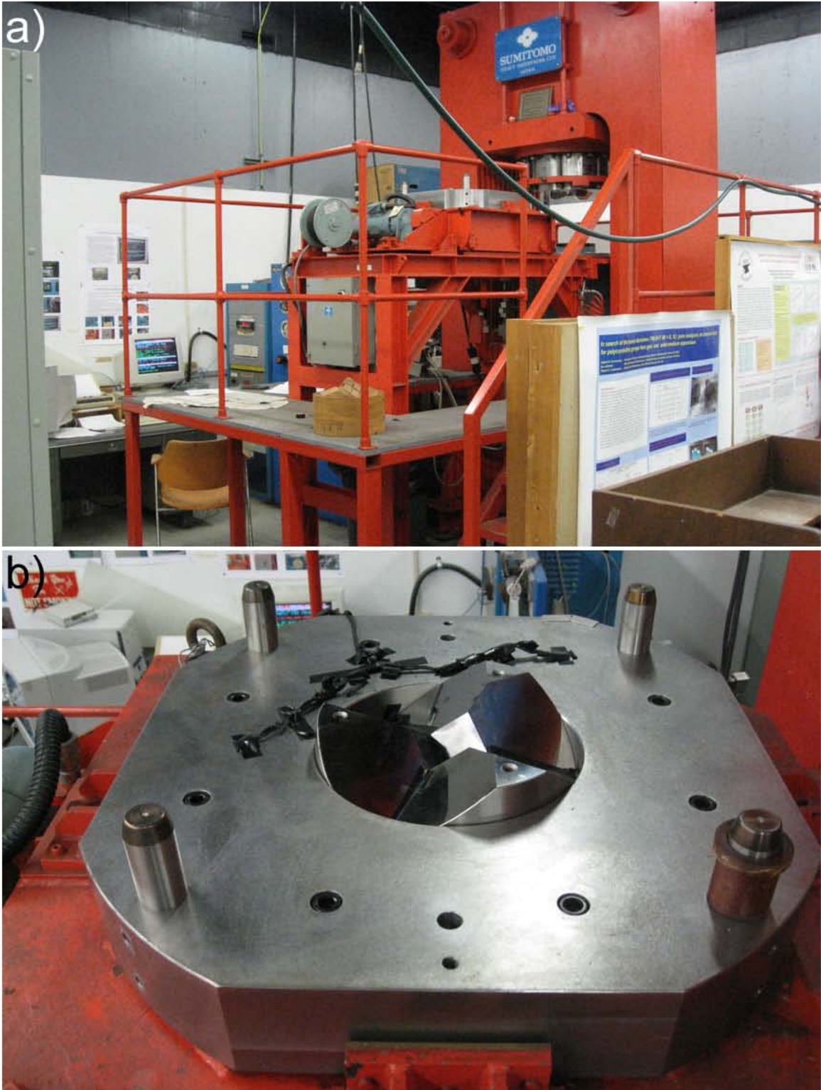
Figure 2.1.2. The Sumitomo Press (USCA-2000): 2000-ton uniaxial split-cylinder apparatus. a) Front view, showing computer controls, catwalk, and press. b) View downward into the base of the press showing where the cubic anvil assembly goes during the experiment.
