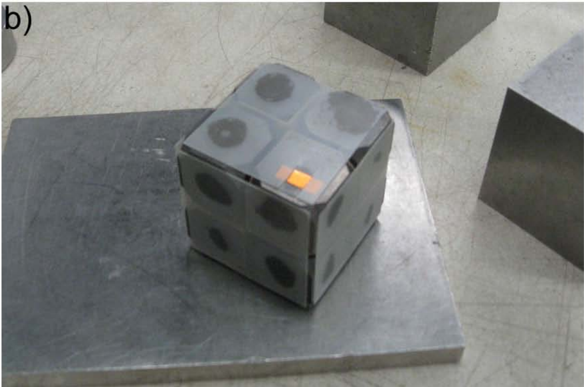
Figure 2.1.6. a) Photograph showing how cubes are assembled such that the pyrophyllite gaskets form a cup for the octahedral cell assembly to be placed into. b) Photograph of all cubes assembled and held in place by the resin sheets. Note the copper strip on the top that allows electrical contact only to the cubes that are in contact with the furnace assembly, while all other anvils are insulated by the resin sheets.
