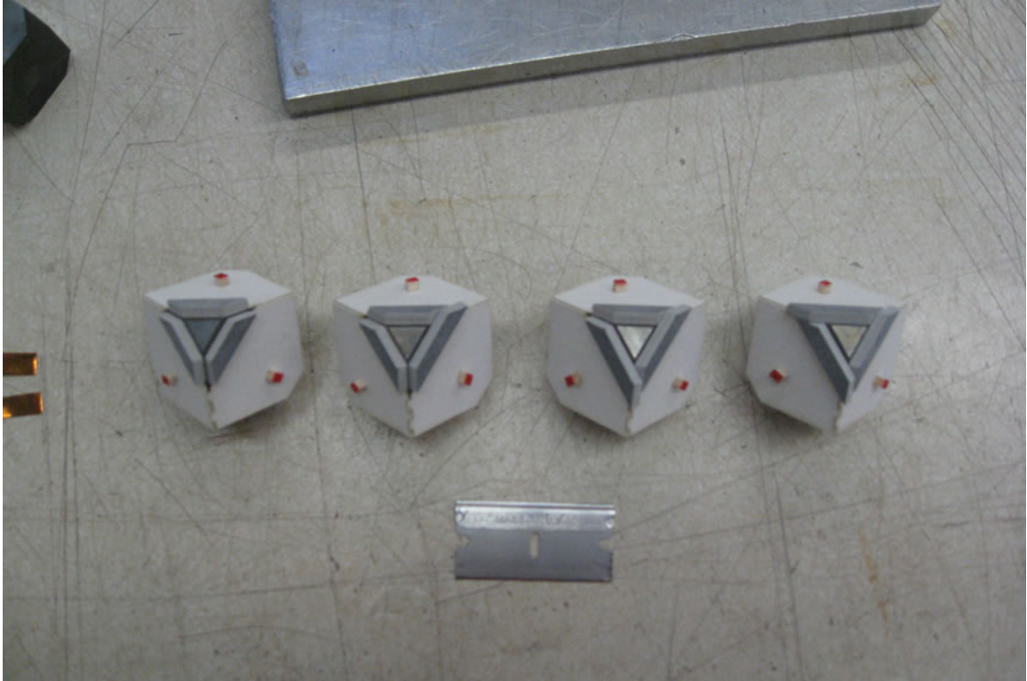
Figure 2.1.5. Photograph of cubes with insulating paper, pyrophyllite gaskets, and balsa wood strip glued in place. Note that the cube on the left has 3 short gaskets, the second has 2 short and 1 long, the thirds has 1 short and 2 long, and the fourth has 3 long gaskets, and that the extra length of the long gaskets always hangs off to the left.
