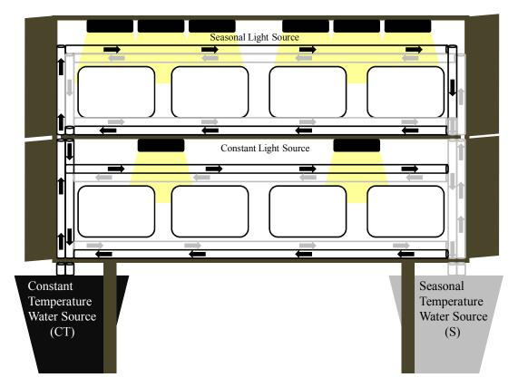
Figure 4.1: Diagram of experimental setup showing the constant and seasonal sea water systems, position of plastic trays containing skates (white boxes), and appropriate light sources. The top level represents the seasonal light scheme while the bottom represents the constant light level.
