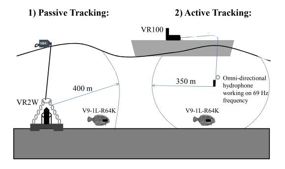
Figure 2.3: Schematic drawing of the two tracking systems (adapted from Yokota et al. 2006). The range for the VR2W was calculated for a 142 dB V9 coded pinger tag assuming calm wind speeds and is subject to change depending on conditions. The range of the VR100 unit was determined by a field test and is also subject to change depending on conditions. Black rectangle on fish represents acoustic tag.
