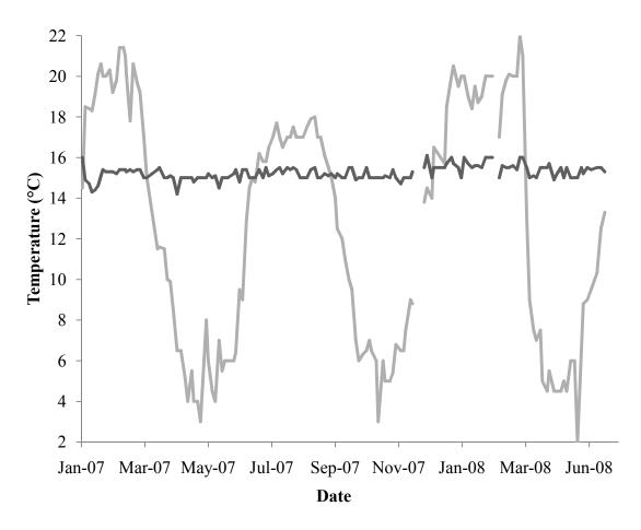
Figure 4.2: Temperature records for the constant temperature seawater system (dark) and the seasonal temperature seawater system (light).
