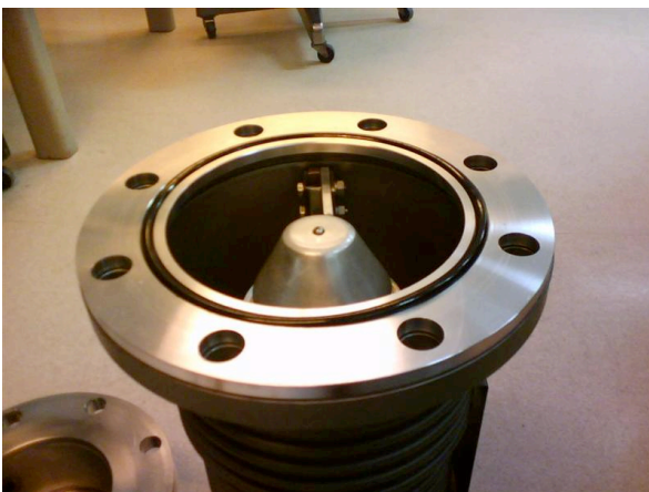
Picture 9. Flange in position with o-ring in place. Pump is ready to be remounted on RIE system.
