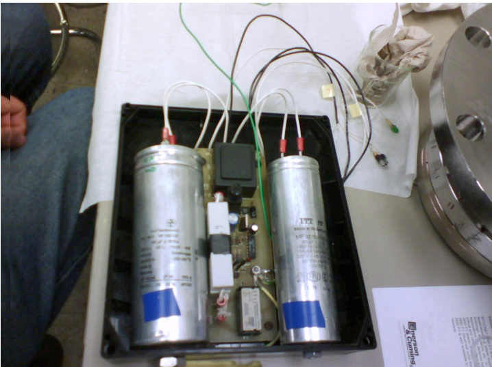
Picture 11. All new wiring, and electronic components reassembled. Starting and running capacitors on the sides.
