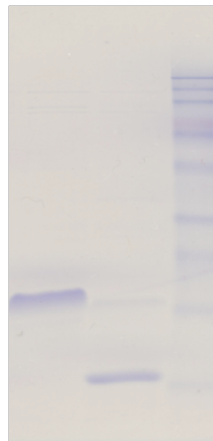
Figure 2.1: SDS-PAGE analysis of ACP conversion. Samples from left to right: apo-ACP, dodecenoyl ACP, and protein ladder (from top to bottom: 170.8, 109.5, 78.9, 60.4, 47.2, 35.1, 24.9, 18.3, 13.7, and 5.7 kDa).
