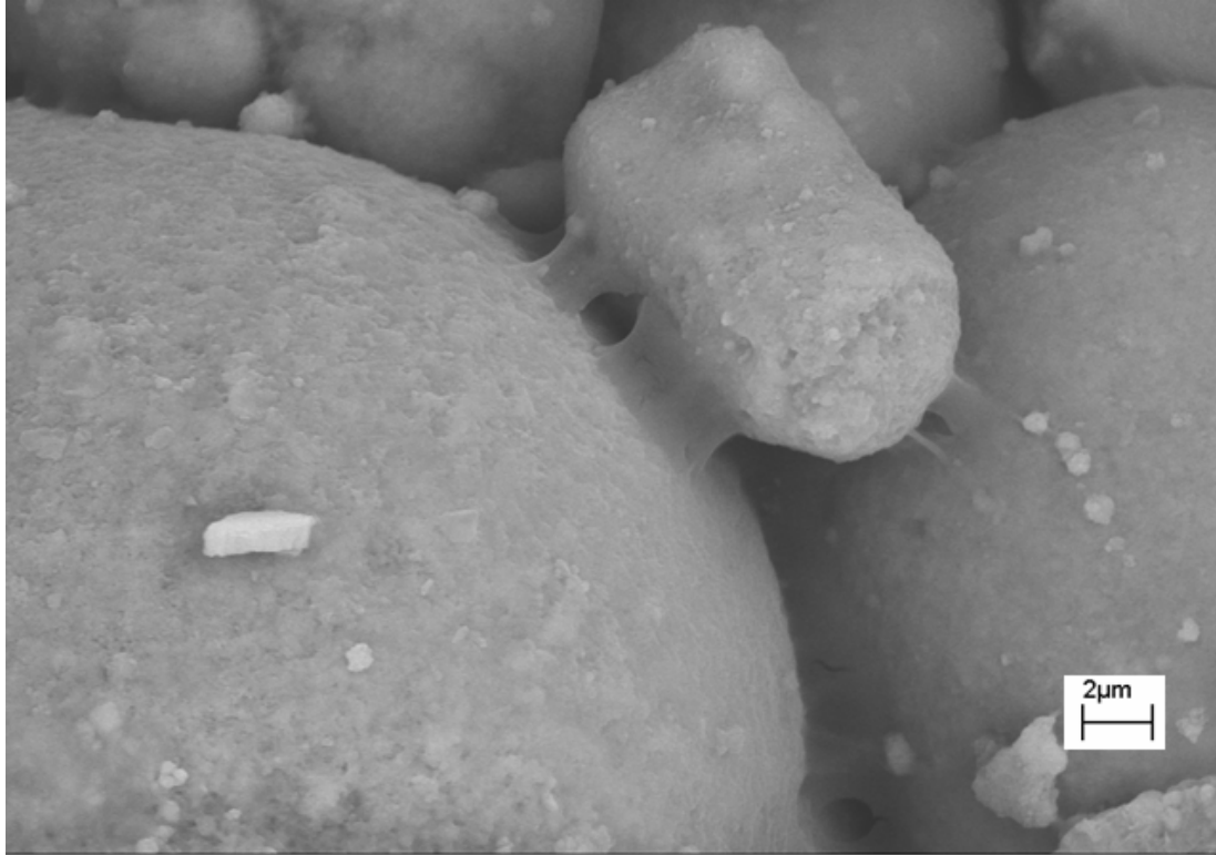
Figure 2.4: SEM micrograph of chitosan/hydroxyapatite composite sample 1.1. Chitosan film can be seen stretched between hydroxyapatite particles.
