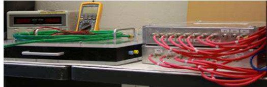
(b) HV Test Boxes for Resistor Chain and Divider
