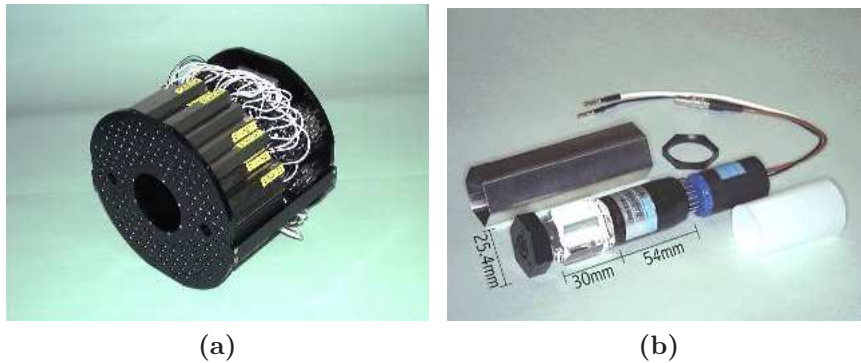
Figure 1.4: The basic components of the BBC. (a) 64 PMTs are mounted to one BBC unit; (b) each single photomultiplier tube (PMT) with a timing resolution of 50ps is of 25.4mm in diameter and has a 30mm thick Quartz radiator.
