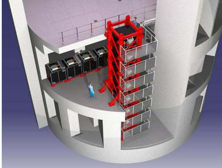
Figure 2.5: A schematic of the INGRID detector. Black boxes are the detector modules arranged in a cross.
