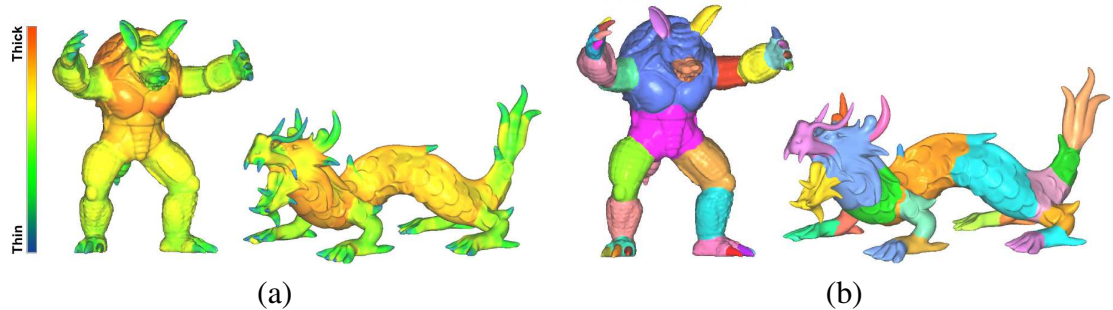
Figure 17: A visualization of the local thickness at each skeleton node in (a), and segmentation results in (b). (Image Courtesy of Au et al. [6])
