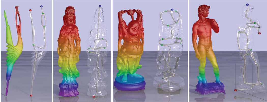
Figure 13: An example of Reeb graph: the pseudo-colored surfaces show the function used for computing the Reeb graph. The transparent models show the structure of the Reeb graph and its embedding. (Image Courtesy of Pascucci et al. [114])
