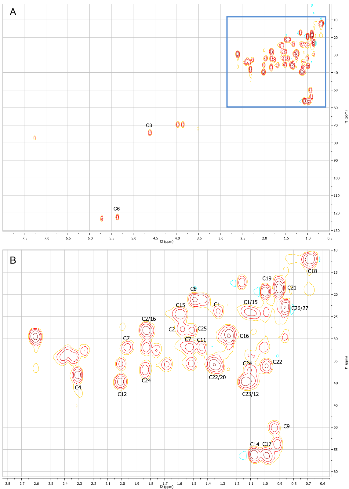
Figure 4-13. ^1\text{H} - ^{13}\text{C} HSQC spectrum (A) and the magnified display (B) of the region boxed in a rectangle in (A) of the cholesterol-derived apolar lipid.
