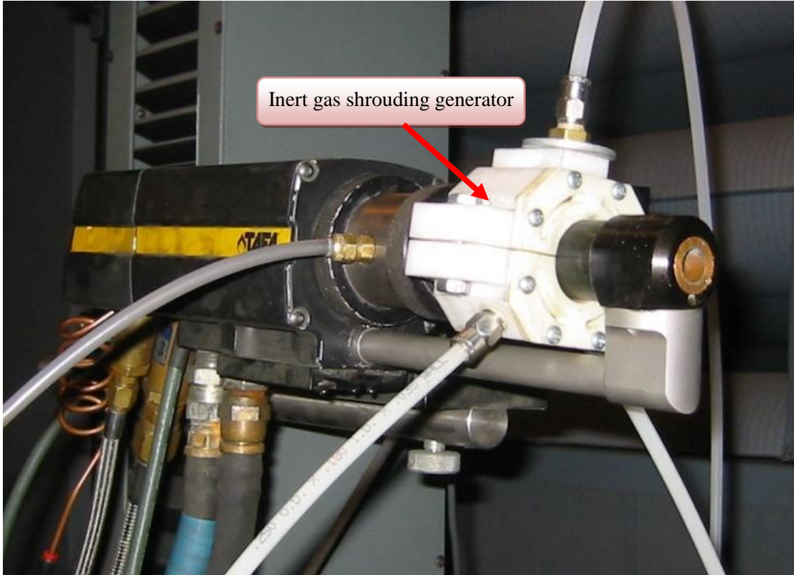
Figure 3.2: HVOF spray gun with inert gas shielding generator
