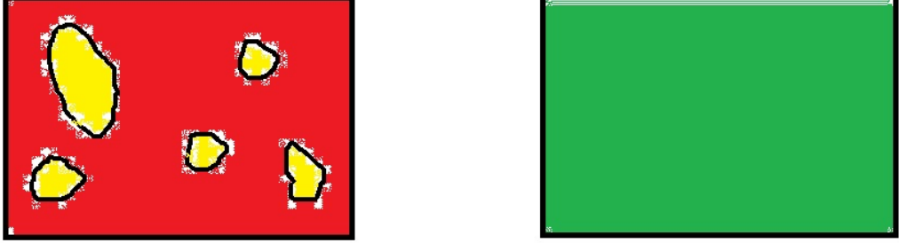
Figure 2: The schematic diagram shows a heterogeneous material (red and yellow) with varying material parameters and a reference medium with constant material parameters (green).
