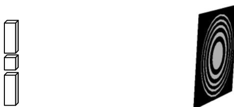
Figure 7-4. The double slit component (left) and the Fresnel zone plate component (right).
