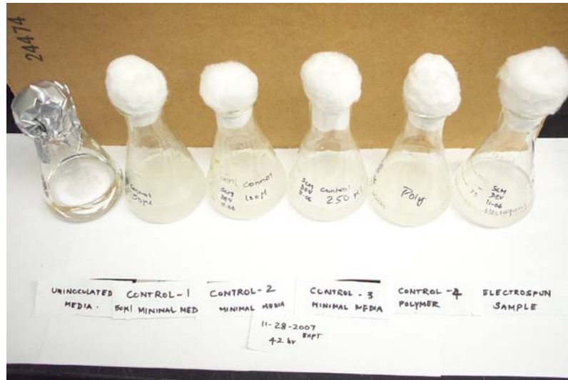
Figure 4.9. A photo of the un-inoculated culture medium and the five inoculated flasks showing the growth of P. fluorescens after 42 hours of growth (data shown in previous Figure 4.7). Controls 1, 2 and 3 are from inoculation of 50, 100 and 250 \mu\text{L} of a fresh culture. Control 4 and Electrospun sample denote flasks inoculated with 100 \mu\text{L} of polymer solution containing the bacteria just prior to and immediately after electrospinning.
