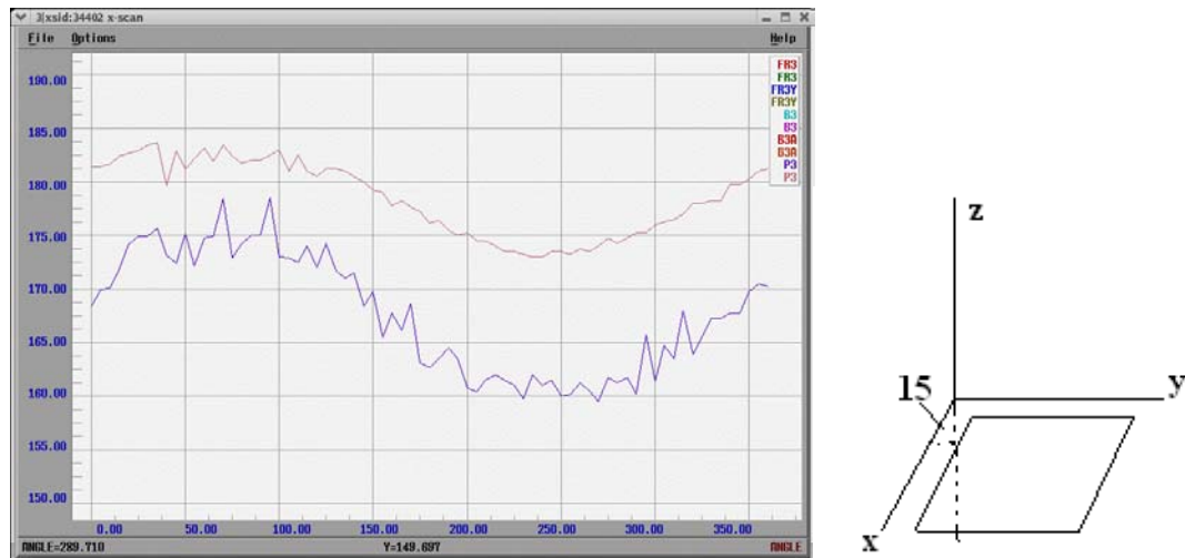
Figure 5.16: Margins of the circuit due to the scan of 360 degrees of magnetic filed. The orientation of the chip to the axis of the magnetic field is also shown as reference
