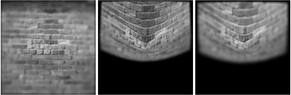
Figure 4.17: Left: Image of a conical object with shift variant defocus blur. Centre, Right: Image of a conical object after a 20^\circ rotation about the x axis and 10 mm translation in the z direction away from the lens with missing pixels and after processing using AIT. Number of missing pixels resolved - 26122
