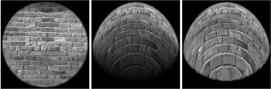
Figure 4.13: Left:Image of a spherical object with shift variant defocus blur. Centre, Right: Image of a spherical object after a 45^\circ rotation about the x axis with missing pixels and after processing using AIT. Number of missing pixels resolved - 68804
