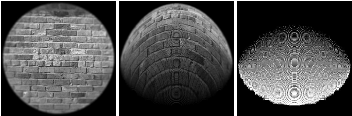
Figure 4.8: Left: Image of a spherical object with shift variant defocus blur. Centre: Image of a spherical object after a 45^\circ rotation about the x axis with missing pixels. Right: Mask image corresponding to missing pixels
