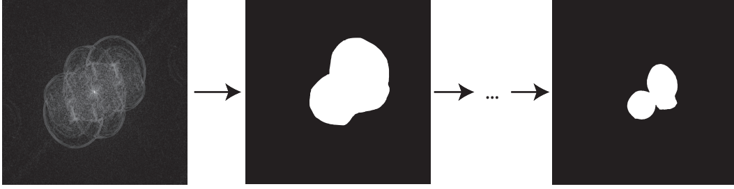
Figure 2.8: From autocorrelation of the object shown on left to first support guess (middle). Usually the support is updated multiple times during the reconstruction process. A good support guess (shown on right for this data set) is crucial for successful reconstruction.
