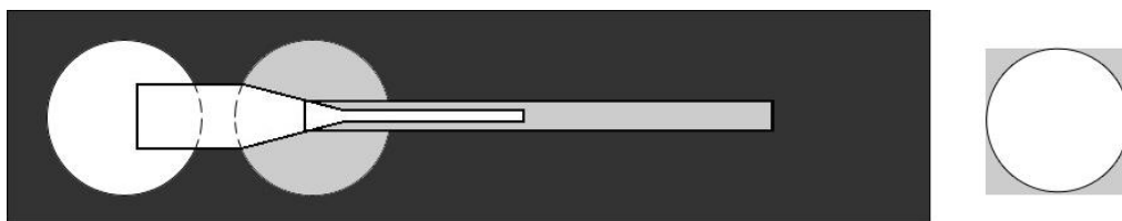
Fig. 4.3 Schematic view of the center injection capillary layout. The cross section view shows its self-centered geometry.
