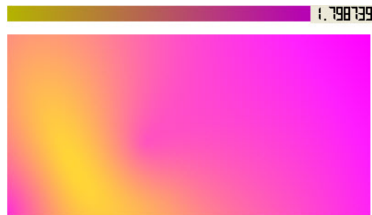
Figure 8.13: The error map for the point constraint of a line segment: yellow points have smaller error than the pink ones for approximation of a line segment.
