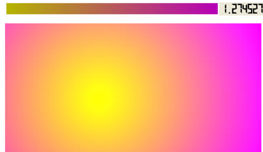
Figure 8.11: The error map for the point constraint of an ellipse: Yellow points have smaller error than the pink ones for approximation of an ellipse.
