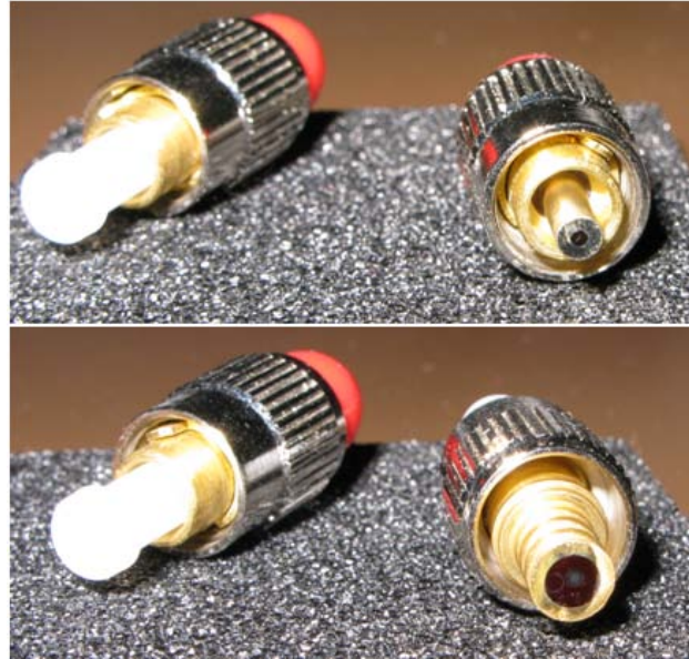
Figure 3.9 CFBs mounted in FCPC connectors (Picture taken on a CFB was experimented without a spacer) Top) Proximal end of the CFB (Laser Pulsing end); Bottom) Distal end of the CFB (MFT transporting end);
