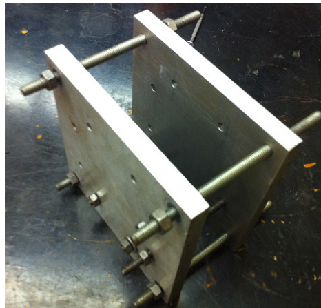
Fig 2.12 An aluminum mold for compressing the conventional foam triaxially
