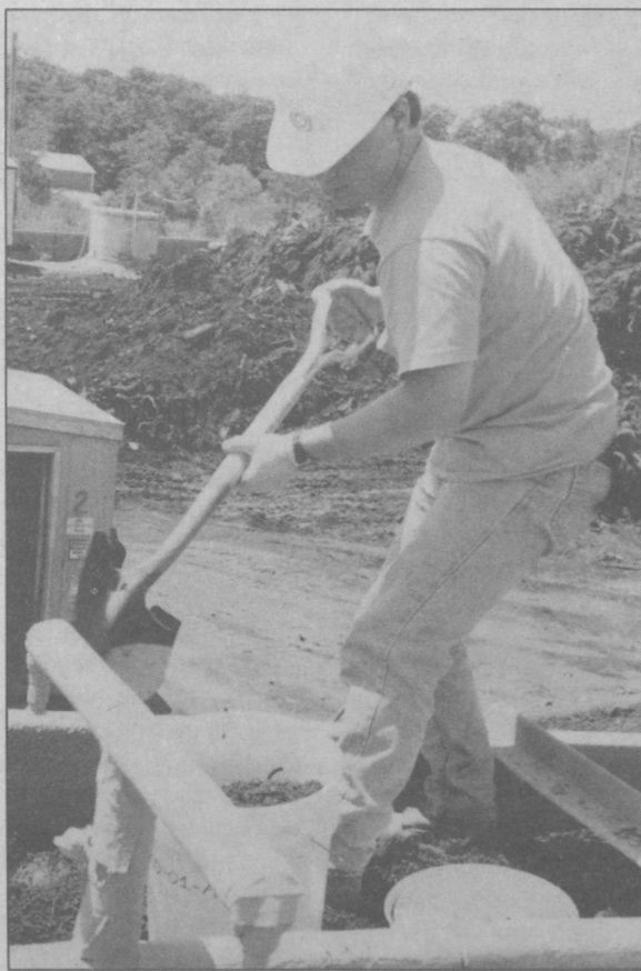
A worker shovels the ash-cement mix being tested at the Waste Management Institute on campus.
