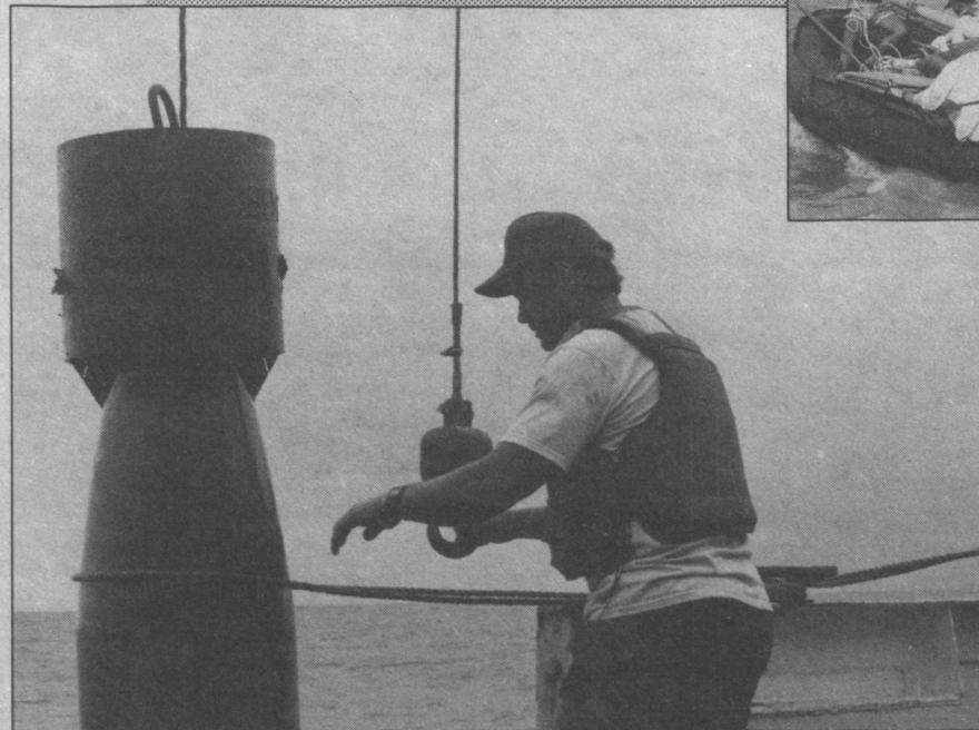
MSRC oceanographer Chuck Nittrouer brings up a piston-coring sample.
