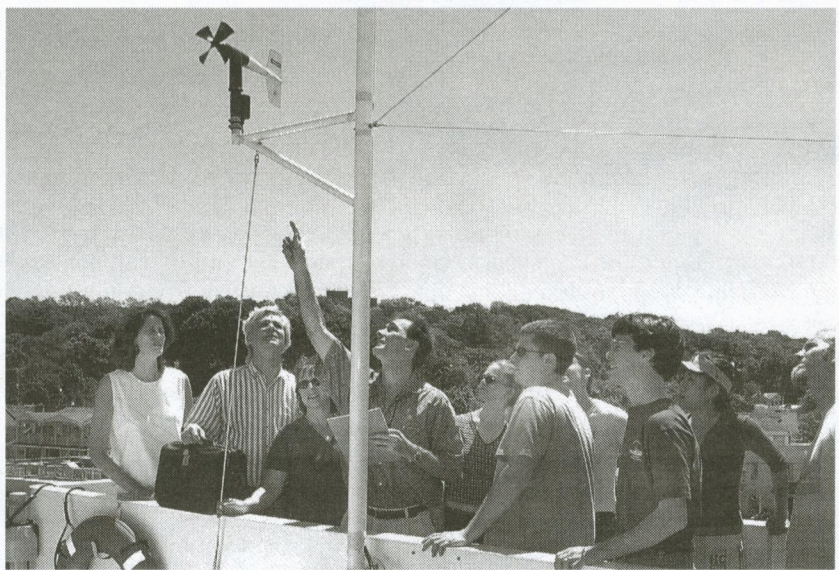
Professor Waliser points at the wind sensor on the PT Barnum 's port bridge wing that provides direction and wind speed. At the top of the mast is the solar radiation sensor.
