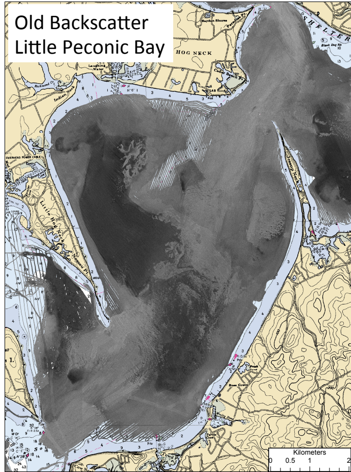
Figure 4: Original backscatter mosaic for the Little Peconic Bay. Mosaic was processed using in-house software at SoMAS. Final mosaic was merged from 5 individual surveys.
