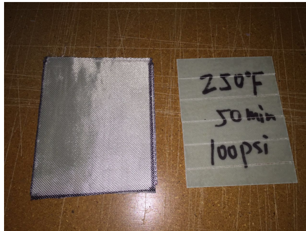
Fig. 2. 3 Flexural test sample
