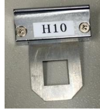
Figure 19: The divergence height limiting slit used throughout XRD analysis. It is the largest slit that can be used; meaning that it allows for all of the sample be irradiated.
