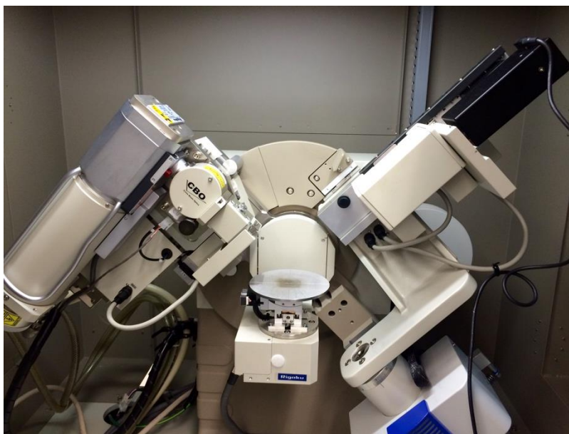
Figure 13: The Rigaku Ultima III's X-ray tube (A), sample holder (B), and an X-ray detector (C).
