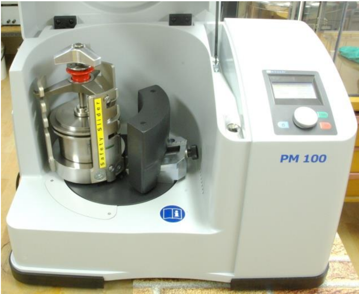
Figure 10: Retsch PM100 Planetary Ball Mill used within a glove box to mill the Al-Si, Al-Zn, Al-Mg, and Al-Zr powder systems [42]. This ball mill only has only 1 grinding station.
