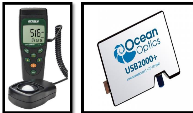
Figure 6. Extech LT 45 light meter for LED lights (left), Ocean Optics USB2000 Spectrometer (right)
