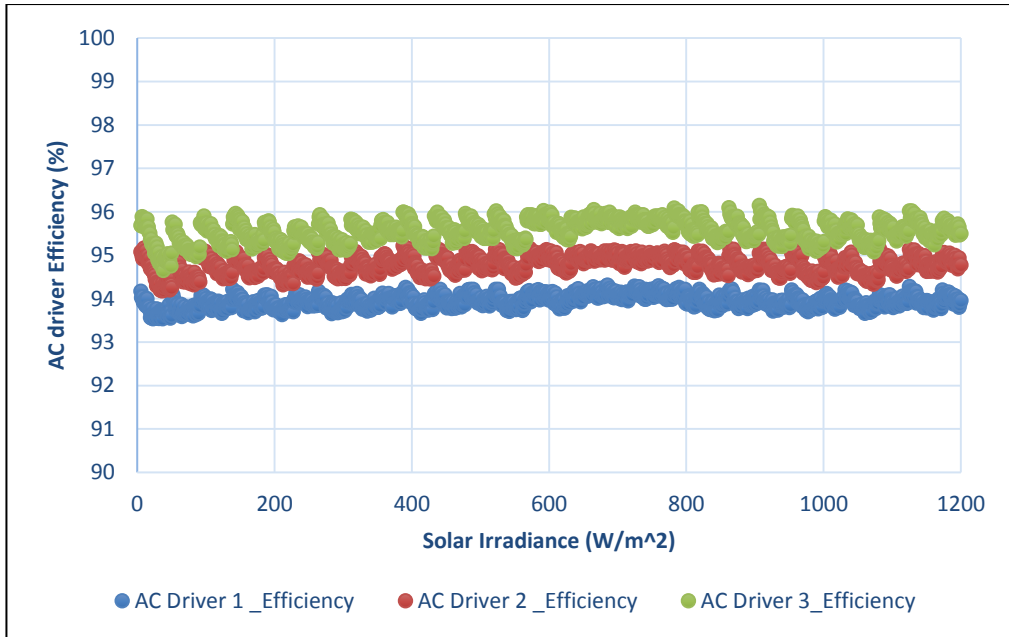
Figure. 6 AC driver efficiencies versus irradiance
