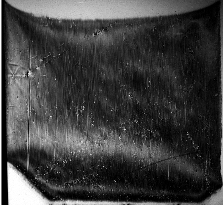
Figure 3.29 Grazing incidence topograph showing TSDs and TEDs.
