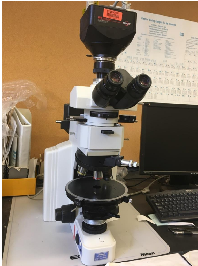
Figure 2.8 Nikon Polarizing Microscope Eclipse E600W POL used for Nomarski optical microscopy.
