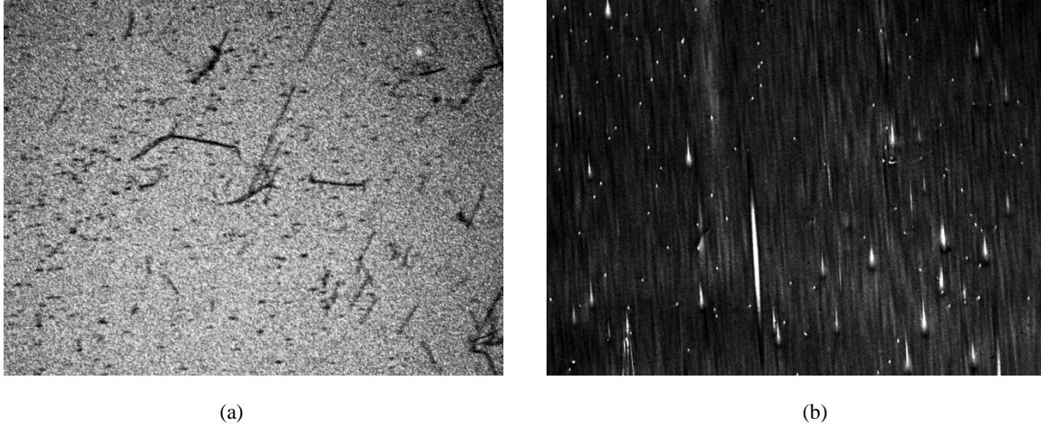
Figure 2.5 X-ray topography images (a) white beam X-ray (b) monochromatic beam X-ray with the area 2.3mm×1.7mm.
