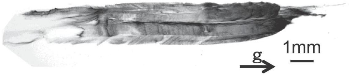
Figure 5.12. SWBXT topograph of fiber 2 showing developing facets
