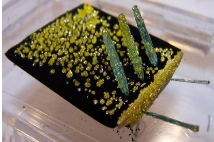
Figure 5.10. Post growth results for the eight hour growth showing three m-plane fibers mounted on top of an uncoated graphite carrier. Two other control fibers protrude from the front of the carrier. Yellow 3C-SiC decorates the surface of the as-grown crystals
