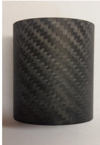
Figure-6 Uncoated carbon composite specimen before the sand particle erosion test
