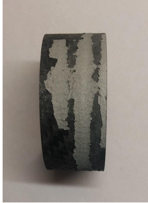
Figure-9 Zinc coated sample after the test
