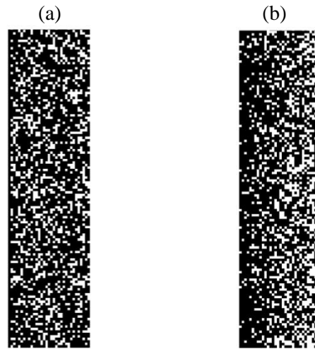
Fig. 5. 17 2D cross section snapshot of the electrode morphologies: (a) pure random, and (b) modified
