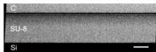
Figure S2. Bright-field, high-contrast cross-sectional TEM micrograph of the SU-8 film (CP-processed) after 10 cycles of ZnO infiltration synthesis. The dark contrast on the upper portion of the film is originating from the infiltrated ZnO. The visible ZnO infiltration depth is ~50 nm with a ~3 nm thick dense ZnO layer on top of the film. C refers to the protective carbon capping layer. The scale bar denotes 50 nm.
