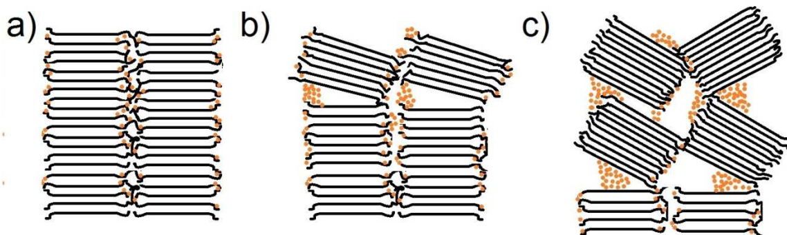
Figure 3- 13 Sketch demonstrating P3HT crystallization induced PCBM phase segregation on blend surface region a) thermal annealing sample b) high pressure scCO 2 sample c) fluctuation ridge scCO 2 sample
