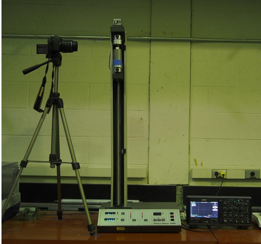
Fig.15. Experimental set-up for tensile and compression test
