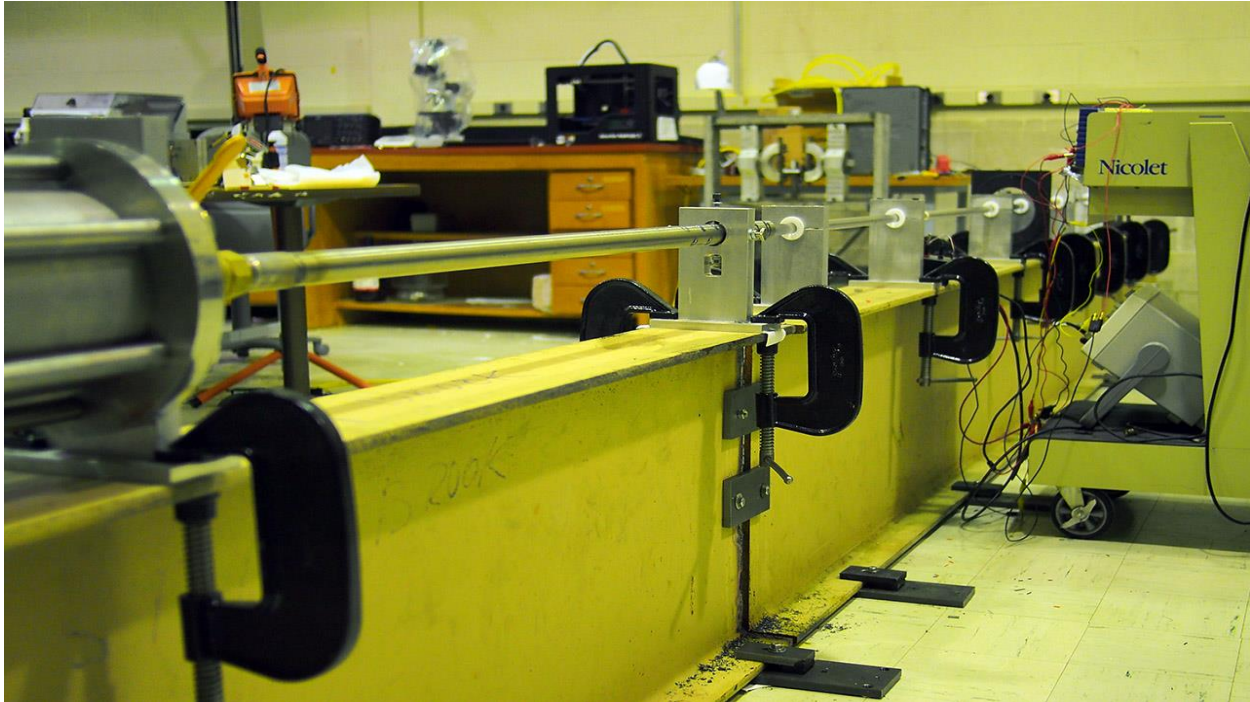
Fig.9. Experimental set-up of SHPB in our lab
