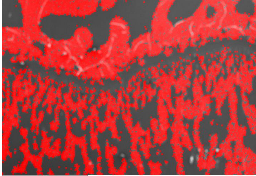
Figure 20: Scanning Electron Microscope image showing elemental distribution of Phosphorus as red dots overlaid on top part of 6AM sample at low magnification.
