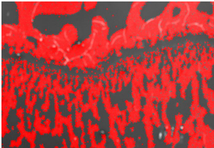
Figure 19: Scanning Electron Microscope image showing elemental distribution of Calcium as red dots overlaid on top part of 6AM sample at low magnification.
