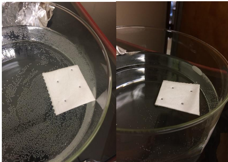
Figure 24: (a) First-day view of commercial PP in buoyancy test (b) After 10 weeks later the view of commercial PP in buoyancy test
