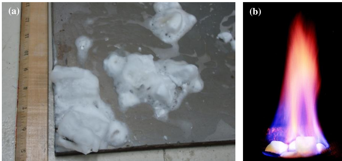
Figure 1.2: (a) CH_4 hydrates formed during experiments in a Parr reactor (taken by Kristine Horvat) (b) A CH_4 hydrate burning (United States Geological Survey) 21
