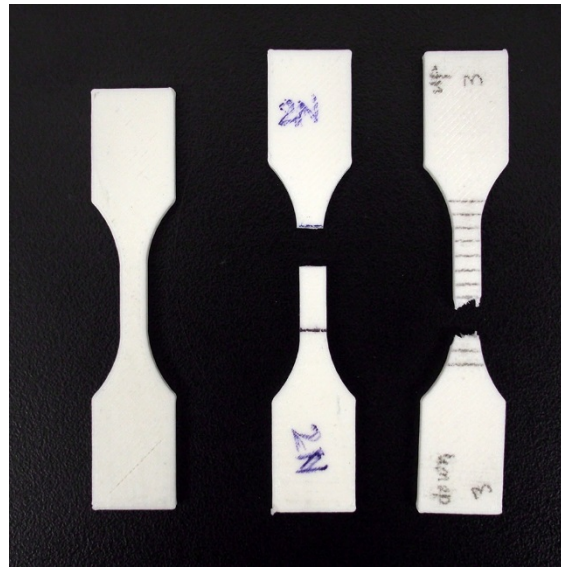
Fig.24 - (a) An original dog-bone specimen, (b) dog-bone sample No.2 (0.05 in/min), (c) dog-bone sample No.3 (0.02 in/min), printed by 3D printer.
