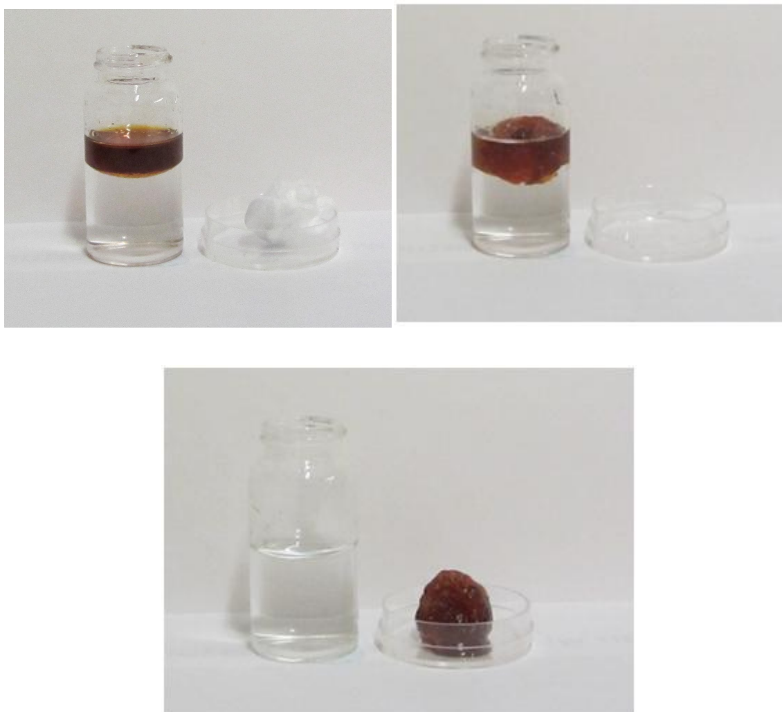
Figure 6.5 Buoyancy and sorption test of No. 6 fuel oil on water by CA fibrous mats.
