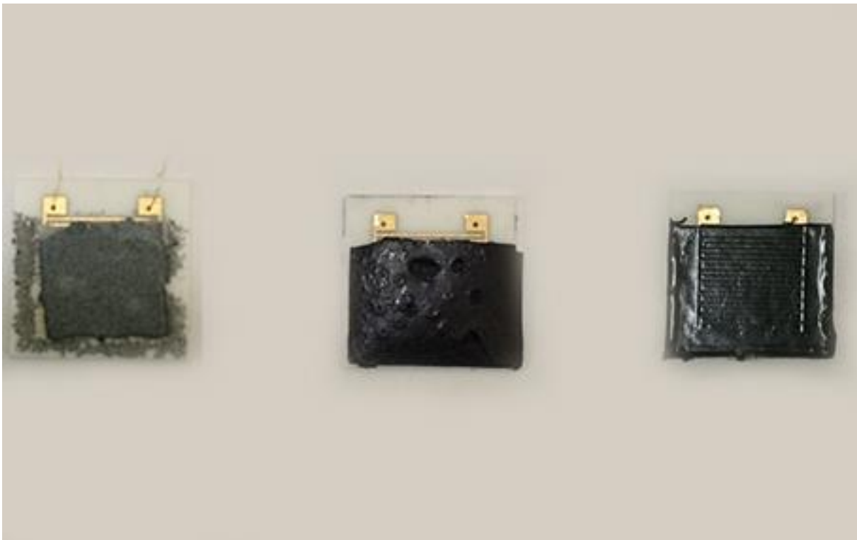
Figure 7 Produced Sensor (From left to right: electrospun, drop coated, spin coated)
