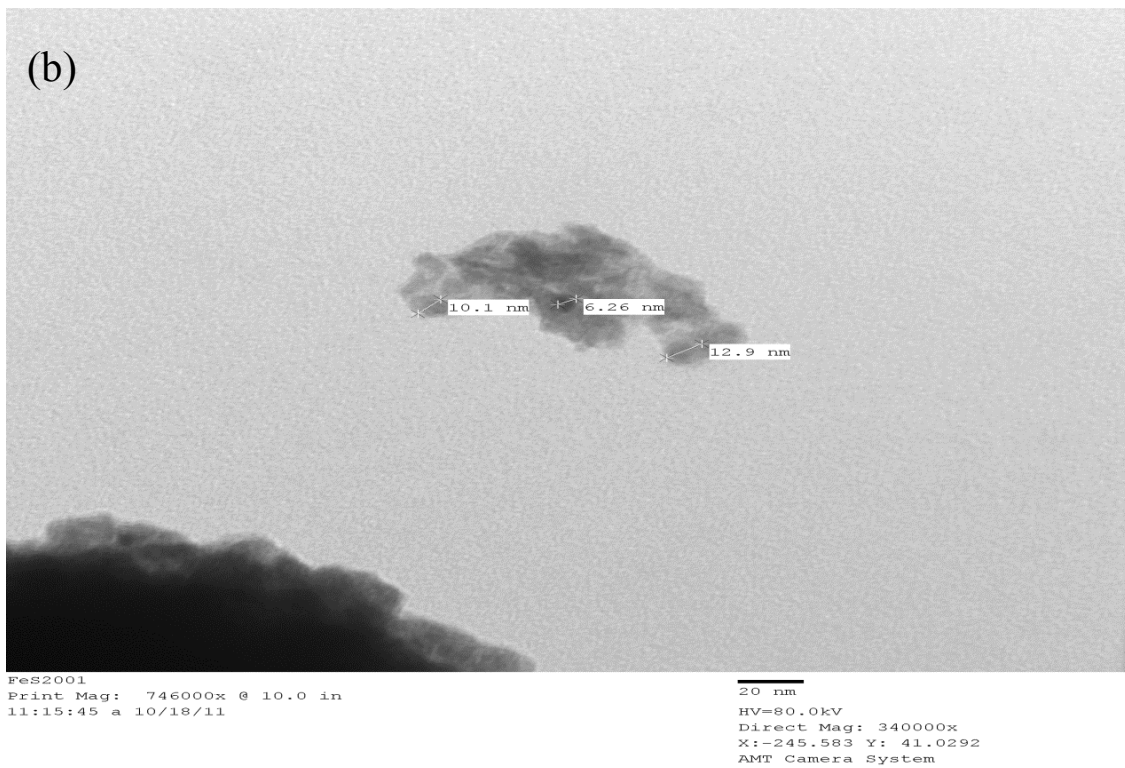
Figure 18 TEM of FeS 2 nanoparticles made in hexadecane
