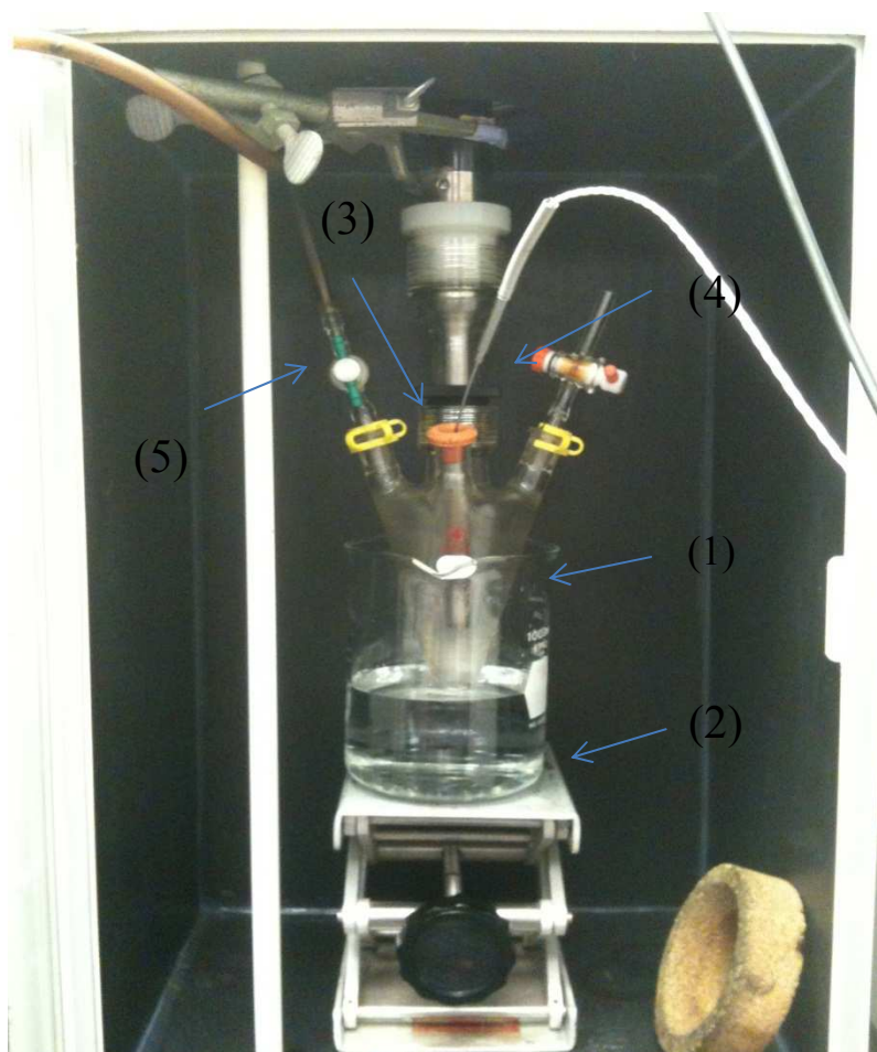
Figure 2 Experiment set up for sonolysis
