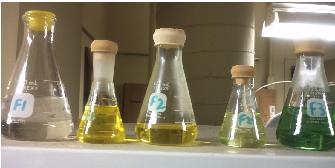
Figure 24 Chemical separation yields the above solvents after column chromatography (starting from left): developing solvent, carotenes, xanthophyll, ChIB, and ChIA. Confirmation of chemical makeup for each extraction was obtained from an NMR study (courtesy of Stony Brook University Chemistry department).
