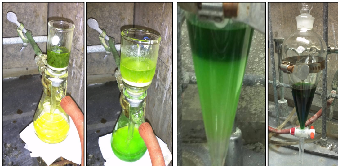
Figure 22a (starting from left) Figure shows the decanting process of methanol, subsequently the methanol solution was discarded. The remaining spinach leaves were re-ground in 25 ml methanol and 35ml petroleum ether. Figure 22b shows second filtration through powder funnel plugged with glass wool. Figure 22c shows lower methanol phase from separatory funnel, removed. Figure 22d (far right) Subsequently, 50 ml distilled water were added to the petroleum ether solution in separatory funnel.
